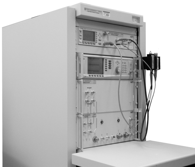
Figure 2.6 LSNA, a sampling-based NVNA.
